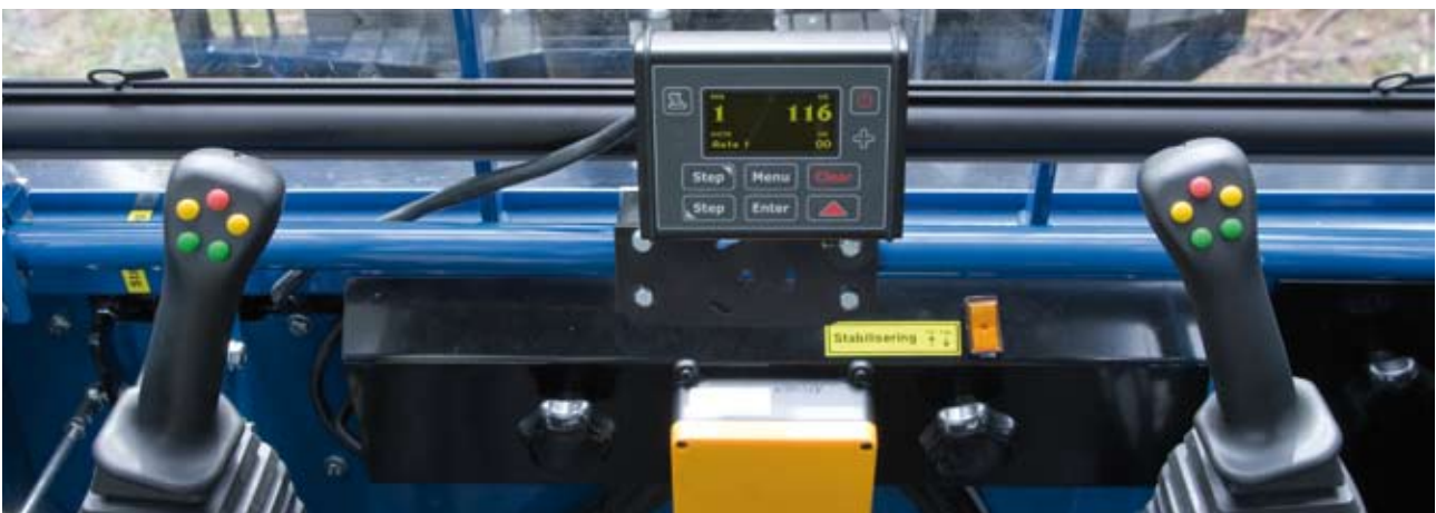
Weight scale system integrated in combi grapple for secure and accurate function. The system register the weight in the combi grapple when unloading harvest and transported biofuel.
