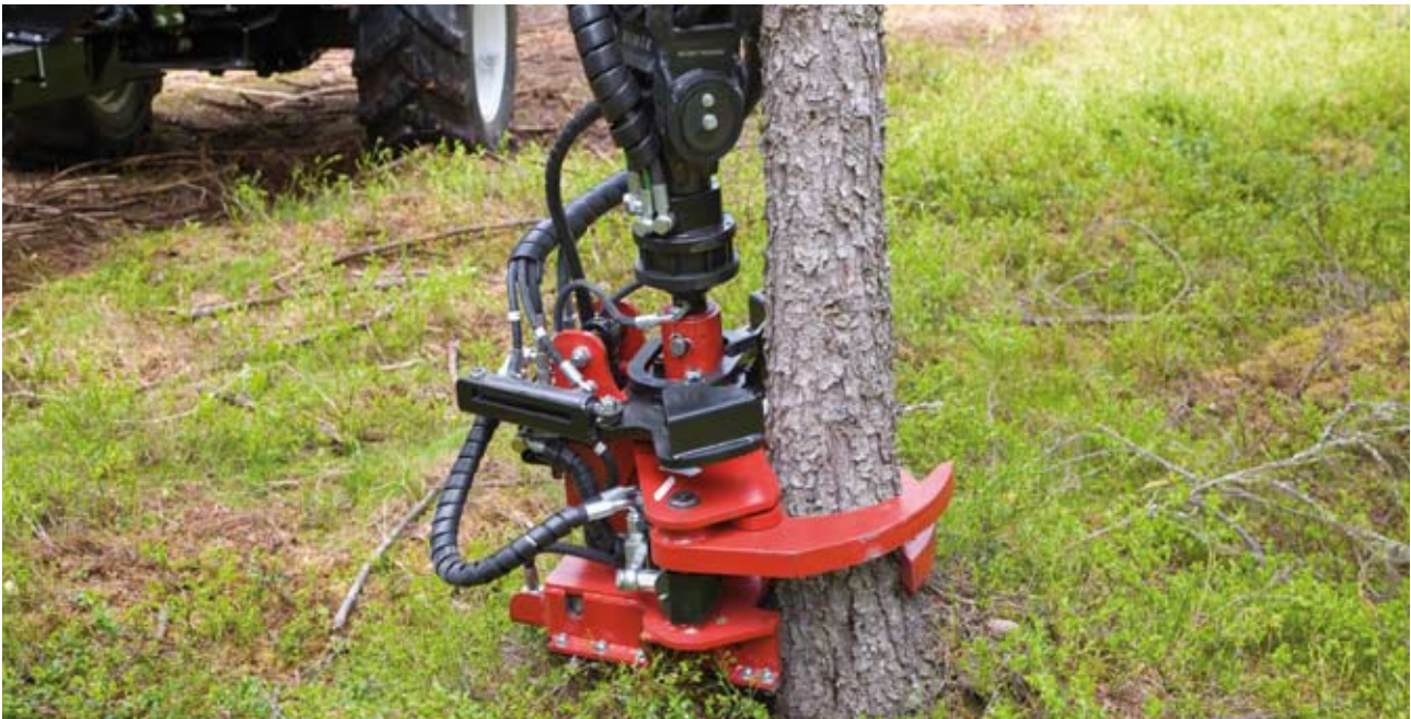
Max cutting diameter: 160 mm. Working pressure: 200 Bar. Rec oil flow: 35 l/min. Weight: 150 kg. Max opening: 670 mm. Cutting force: 8.000 kg.
