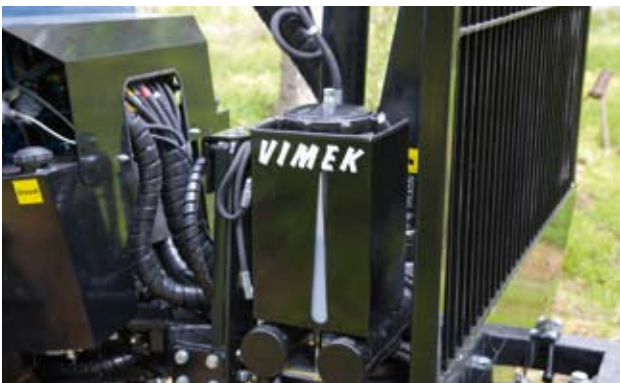
Stump treatment. Unique solution integrated in combi grapple Vimek 160.
